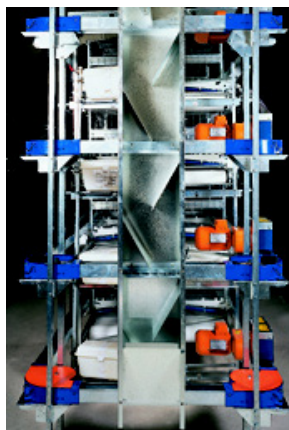
Cascade feed column prevents feed bridging
