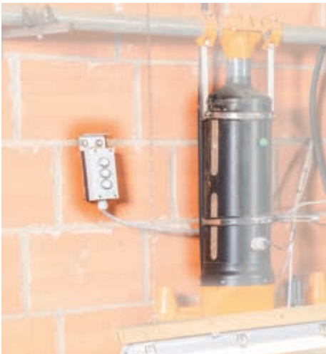
Manual feed dispensing (optional): inspection window in the hopper to check the feed level
