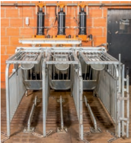
An anti-resting bow stops the sow from remaining in the station for longer than necessary
