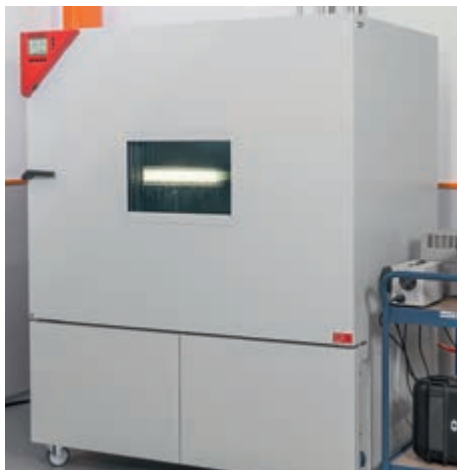
Environmental test chamber
