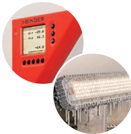
AuroraLED ceiling lamp, tested under temperatures of -25 °C
