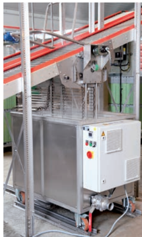
Cleaning unit: for a maximum conveyor width of 750 mm
