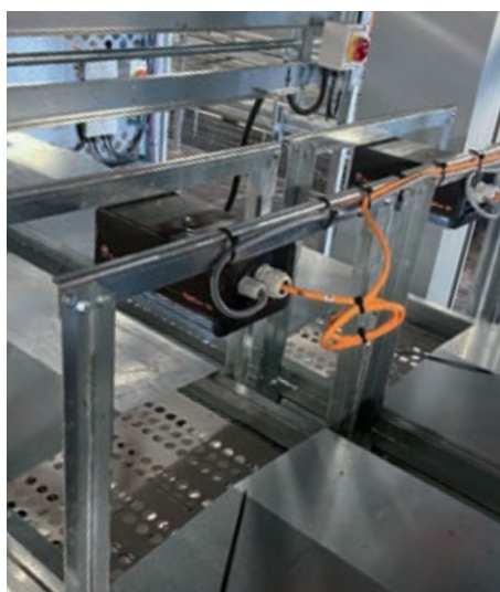
Installation above both longitudinal belts of a NATURA Step XL aviary, directly behind the nest
