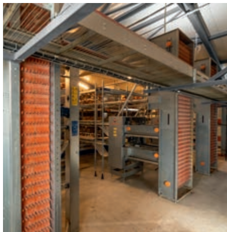
EC elevator with integrated system egg collection
