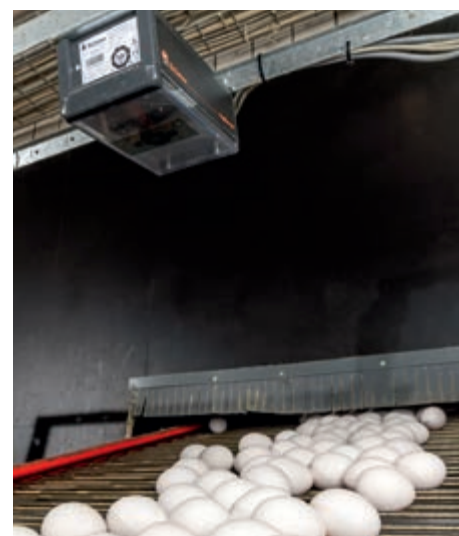
EggCam 3D above the cross belt
