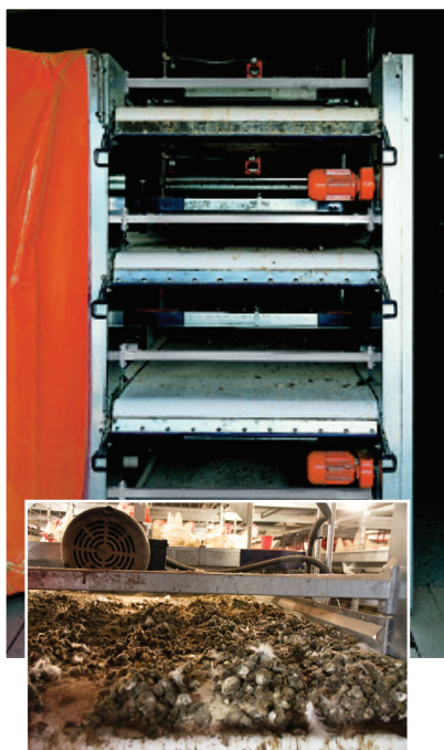
Manure removal end set with manure chute
