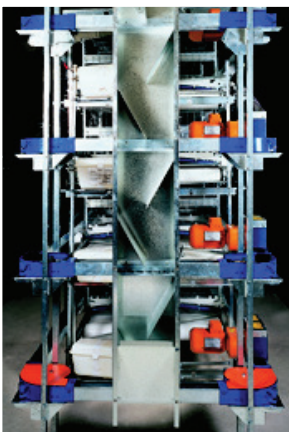
Cascade feed column prevents feed bridging
