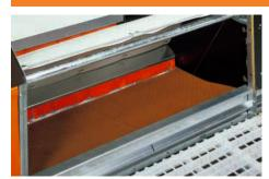
The egg belt is located in the center, allowing the eggs to be laid directly in front of the belt. This design ensures the shortest possible roll-off distance for the eggs, minimizing the amount of cracked and checked eggs.
