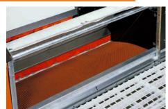
Before the divided nest floor completely closes, it is raised slightly in the center, providing a gentle egg roll-off onto the center egg belt.
