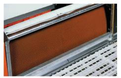
The nest floor is raised completely, allowing any dirt to drop off the nest insert, and closes off the nest to **prevent hens from entering and brooding inside**.
