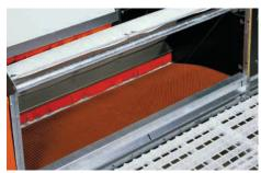
Before the divided nest floor completely closes, it is first raised in the center slightly, which **provides a gentle egg roll off onto the center egg belt**.
