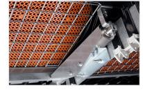
NESCA consists of a bottom wire mesh which rests on four load cells, which transmit their results to the production computer via a weighing module
