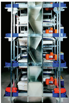
Cascade feed column prevents feed bridging
