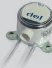
DOL 18 is a negative-pressure sensor that actively measures the pressure in the barn, emitting a 0-10 V signal. Power for this sensor is supplied by ViperTouch.
