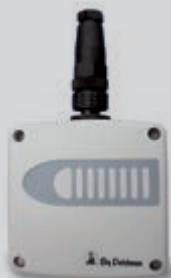
The DOL 19 sensor measures the carbon dioxide concentration of the house air. Its high-quality infrared measuring cell is able to detect CO<sub>2</sub> in a range from 0 to 10,000 ppm. It is thus possible to control minimum ventilation based on the CO<sub>2</sub> concentration.
