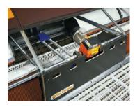
The drive unit for opening and closing the nests consists of a gear motor and a winch. Depending on the length of the nest row, it is located in the center or at the beginning of each row, providing high functional reliability.
