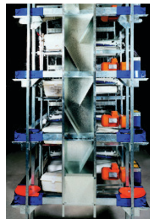
Cascade feed column prevents feed bridging
