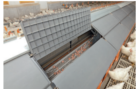
Extra wide plastic perforated egg belt keeps eggs clean and safe
