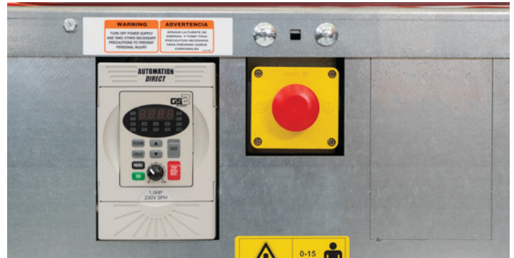
Variable speed front mounted control with reverse and emergency stop
