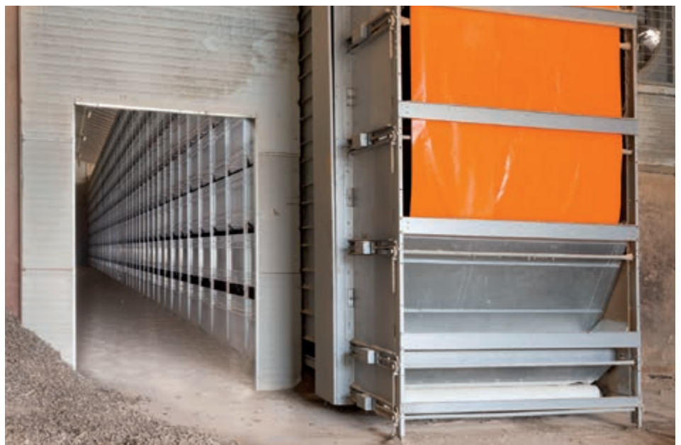
OptiSec manure drying tunnel with 16 tiers
