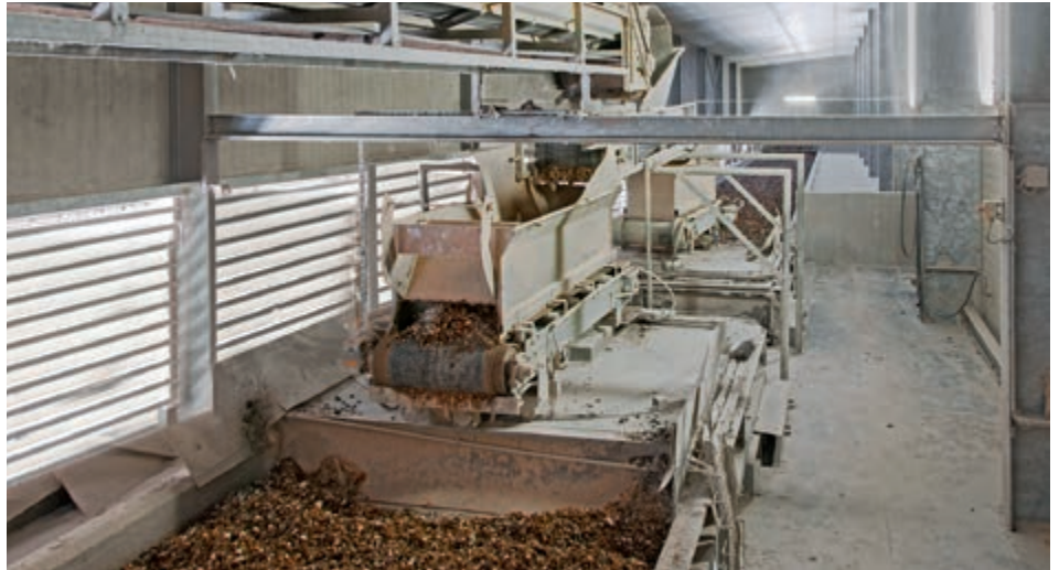
Filling station: Two OptiPlate dryers, installed front-to-front, are supplied by one conveyor belt
