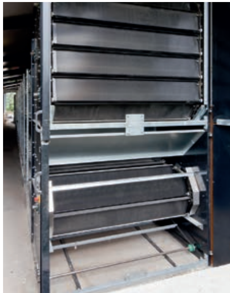
Open OptiPlate with scraper floor
