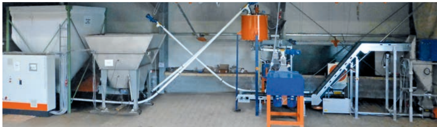
Pellet plant BD PelletFix with two mills and a capacity of 500 kg/h
