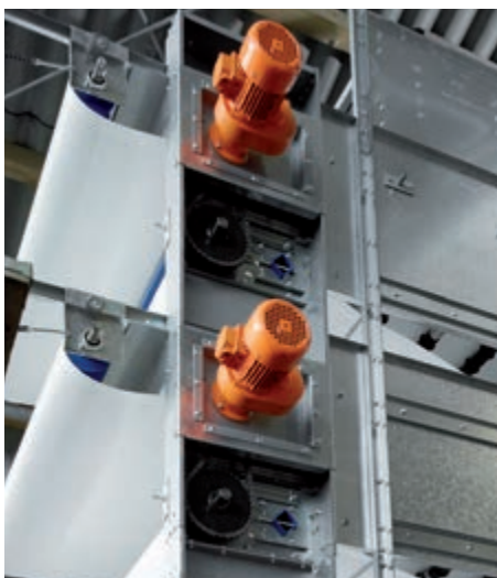
Standard manure belt drive and auger idler in each tier
