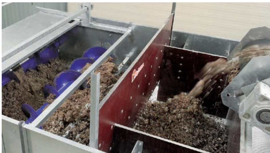
The distributing augers fill the belts evenly
