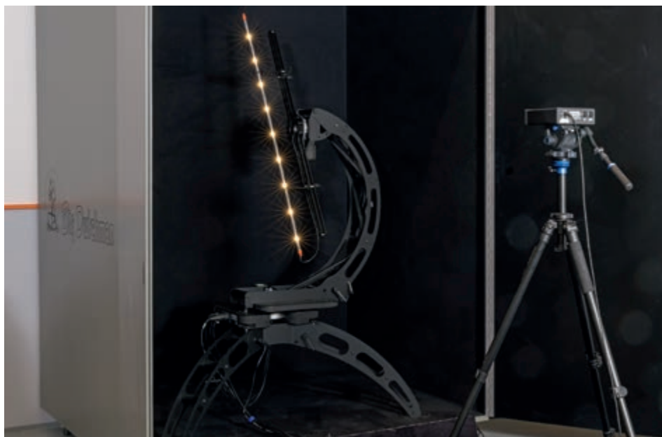
Goniometer – testing our FlexLED lamp
