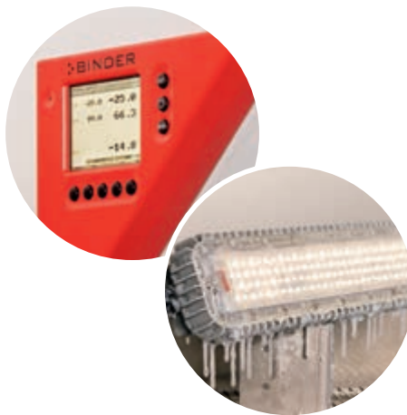
ZeusLED ceiling lamp, tested under temperatures of -25 °C
