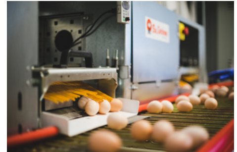
EggTrax egg transfer system helps to clean eggs, and keeps them safe during the transition from the egg belt to the cross conveyor
