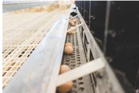
Perforated black plastic egg belt keeps eggs clean and safe. The plastic belt is easy to clean and sanitize.
