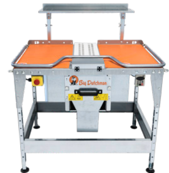
EggTrax egg transfer system helps to clean eggs, and keeps them safe during the transition from the egg belt to the cross conveyor
