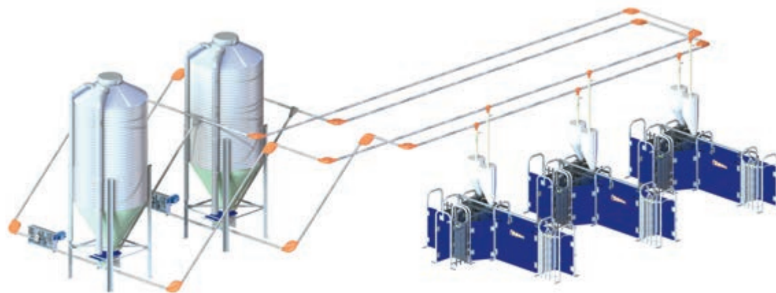
Functional diagram of a CallMatic pro for dry feeding, used of two types of feed
