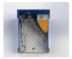
Installing the BDSWING as a diagonal crate is a great option when retrofitting your existing farrowing barn. This allows for a longer crate in a smaller pen, and the SWINGSIDE provides for easy in, easy out.
