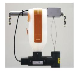
EASYSLIDER is a computer controlled dosing device for farrowing pens mounted underneath the volume dispenser. The sow can choose for herself when and how much she wants to eat, and merely has to actuate a pendulum inside the feed pipe, which releases a portion of feed.
