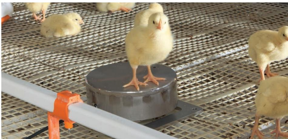
**IncasCompact** is a poultry scale developed by Big Dutchman for broiler weighing in AviMax production systems. It is made of stainless steel and the circular weighing platform has a diameter of 15 cm. IncasCompact is simply positioned on the cage floor where it catches with its two feet. Thanks to its compact design it can also be used as a mobile bird scale.
