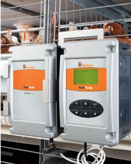
**ComScale** is a stand-alone weighing computer which can be installed stationary in the service room or it can be used as a battery-powered mobile version. ComScale is equipped for the connection of the poultry scales Swing 20 and 70 as well as Incas 2 and IncasCompact.
