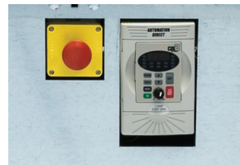
Variable speed front mounted control with reverse and emergency stop
