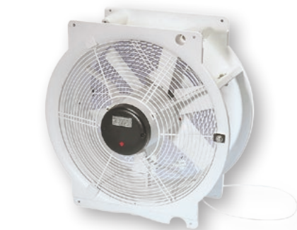
6E50 circulation fan Air capacity: 6400 m³/h, code no. 40-20-1095 Throwing range: approx. 25 m
