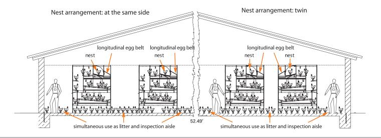
The **NATURA70** has no bird-free inspection aisles, allowing the hens to use the entire house surface as a scratching area, giving the **NATURA70** higher bird capacities than the **NATURA60**. To achieve optimum bird numbers, the scratching area can be split in a longitudinal and transverse direction, which can be repeated depending on house dimensions.
