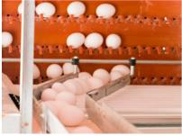
Big Dutchman's EggCellent, patent pending egg elevator uses an innovative design to provide high volume egg collection with less adjustments and maintenance while providing protection for the egg, minimizing cracks and checks.
