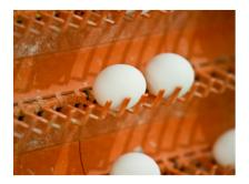
The EggCellent's unique egg conveying chain is made of interlocked plastic module parts, which will not stretch and requires no lubrication. These chain modules feature integrated soft padding for impact protection, providing gentle egg transport.
