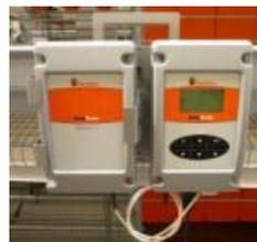
In connection with the retainer and the battery set, it is possible to use ComScale as a mobile weigher. Thus, a quick change between the compartments of a layer house can be realized. The mobile version can also be installed next to a Swing-weigher by means of a chain in the house. Then it is not necessary to provide a connection line to the service room.
