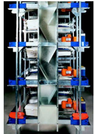
Cascade feed column prevents feed bridging
