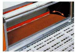
Before the divided nest floor completely closes, it is first raised in the center slightly, which provides a gentle egg roll off onto the center egg belt.
