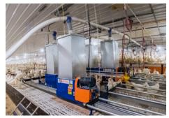
Feed is transported from the feed bins to the feed hoppers inside the barn, and distributed with the CHAMPION® CHAIN FEEDING SYSTEM.
