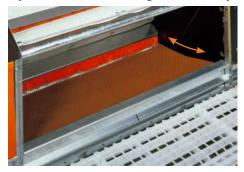
The egg belt is located in the center, allowing the eggs to be laid directly in front of the belt. This design ensures the shortest possible roll-off distance for the eggs, minimizing the amount of cracked and checked eggs.
