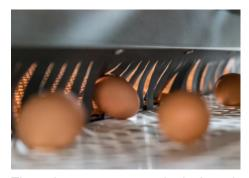
The colony nest system is designed with the egg in mind. The egg has a safe and gentle rollout onto the egg belt from the nest.
