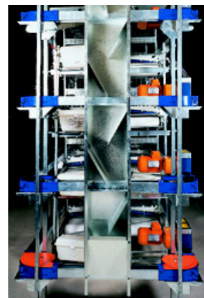
Cascade feed column prevents feed bridging
