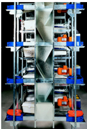
Cascade feed column prevents feed bridging
