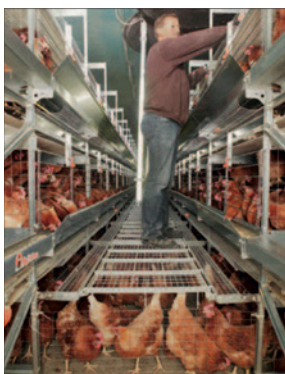
Raised inspection aisle allows for easy inspection of nests and longitudinal egg belt
